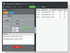
The Console displays the entire verification process on one screen. Data fields change color to show the progress of stability and deviation for each logger. A status window lists each step and indicates where the system is in the process.
