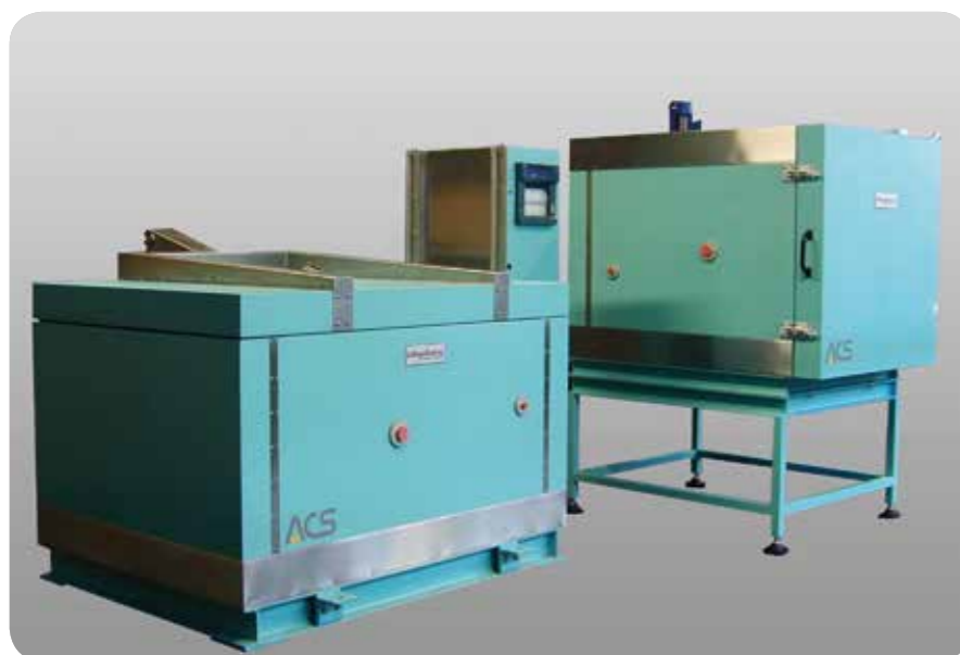
Liquid nitrogen freezers, for temperatures down to -180°C, horizontal and vertical versions.
